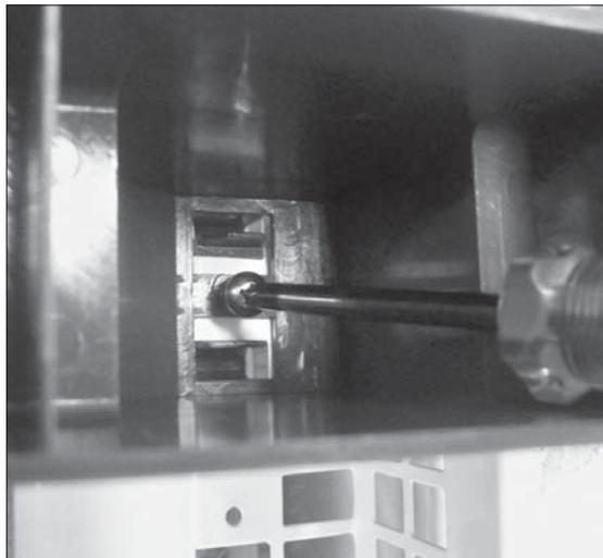
With a small Phillips-head screwdriver, take the provided screw and secure the wheel set into place. Example shown in Figure E.
